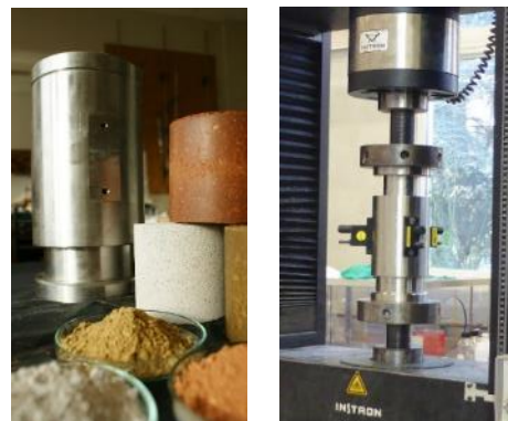
Fig. 17: Compaction mould and vibrators set up on the mould under the loading frame.
