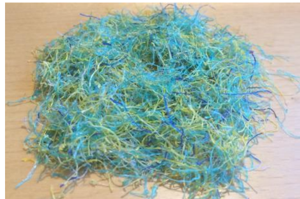
Fig. 3: R-PE fibres from discarded fishing nets after being cleaned in tap water
