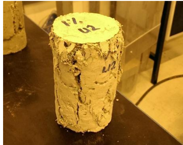
Fig. 9: Adobe cylinder with addition of 1.0\text{wt}\% R-PE after compression test
