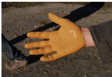
Fig. 4: The glove test practiced on the workplace: the slip is properly designed if some remains on the hand.
