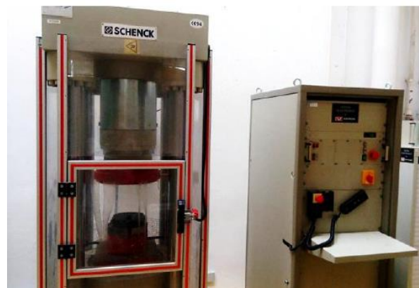
Fig. 2 : INSTRON machine for compressive strength.
