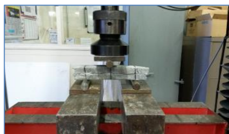
Fig. 6: Flexural test of two 3D printing layers
