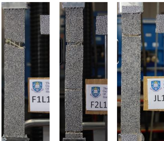
Fig. 48: Typical failure modes of F1-, F2- and J-TRM coupons.
