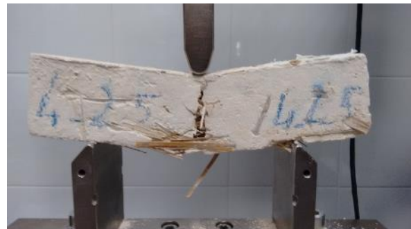
Fig. 55: TPB test of a characteristic short fiber 2 % reinforced specimen.
