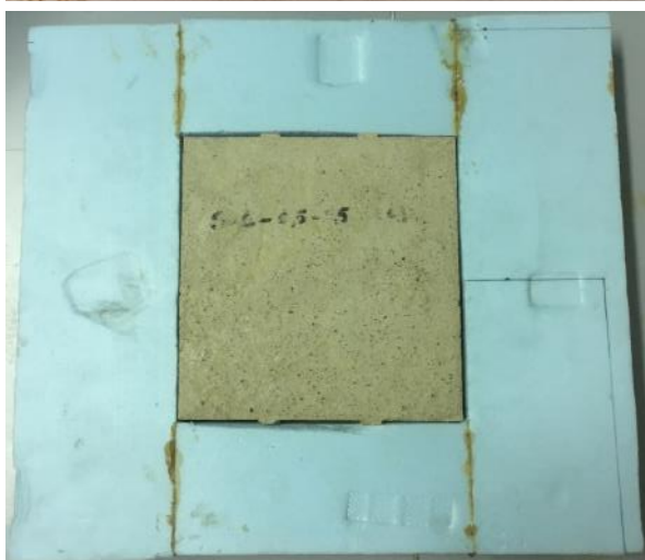
Fig. 4: Samples for thermal conductivity measurement, before and after insertion on guard ring.
