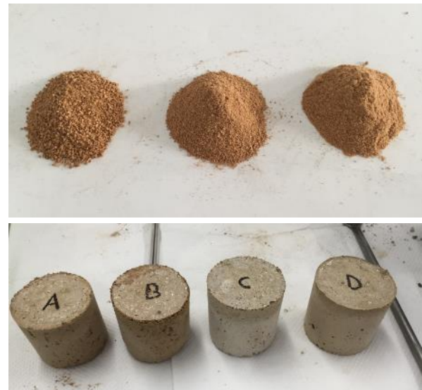
Fig. 2: Up: Cork grainsize from left: 1, 0.5 e 0.25 mm. Down: Preliminary samples for mixing grainsize.
