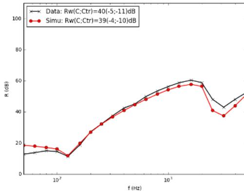
Fig. 7: Comparison between measurement and simulation of the sound reduction index  $R$  of a 72-48 partition wall with 45mm hemp wool filling
