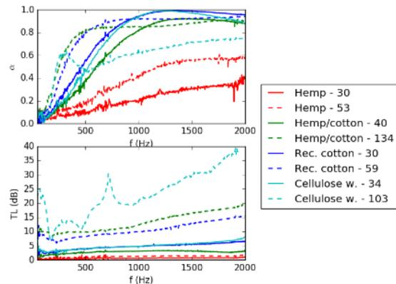
Fig. 1: Acoustical properties of loose fibres
