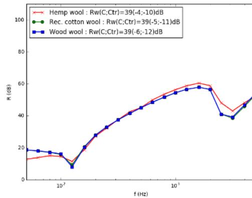
Fig. 11: Simulation of the sound reduction index  $R$  of a 72-48 partition wall with various wools filling
