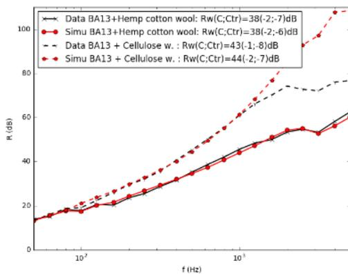
Fig. 10: Comparison between measurement and simulation of the sound reduction index  $R$  of a ceiling with loose fibres (hemp/ cotton fibres and cellulose wadding) insulation
