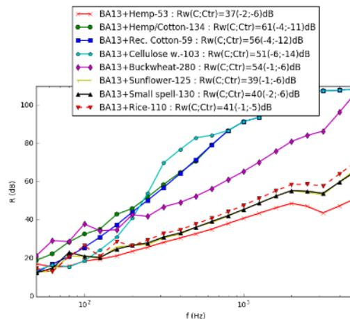
Fig. 12: Simulation of the sound reduction index  $R$  of a ceiling with loose fibres or aggregates insulation
