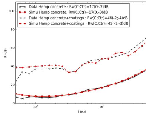
Fig. 8: Comparison between measurement and simulation of the sound reduction index  $R$  of a hemp concrete façade wall without and with coatings
