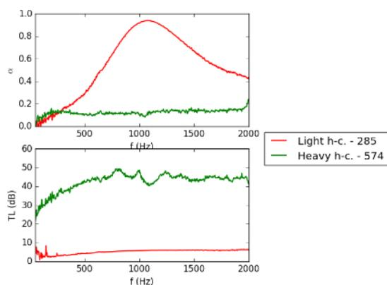
Fig. 4: Acoustical properties of hemp concretes
