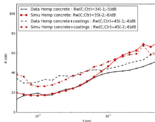
Fig. 9: Comparison between measurement and simulation of the sound reduction index  $R$  of a hemp concrete separation wall without and with coatings
