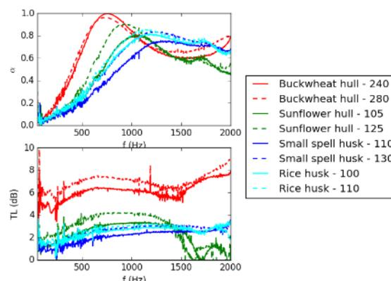
Fig. 2: Acoustical properties of loose husks and hulls
