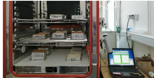
Fig. 67: Experimental bench for MBV measurement.
