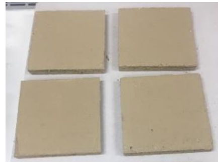
(b) UoB clay specimens after demoulding
