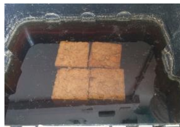
Figure 70 – Rapeseed VMA samples during a full immersion weathering test
