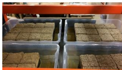
Figure 71 – Samples partially submerged during a partial immersion test
