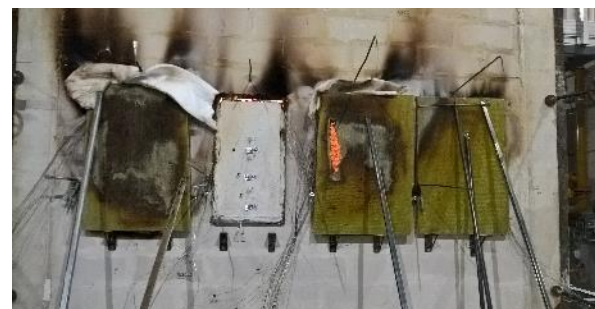
Fig. 5: Unexposed side after 180 min.
