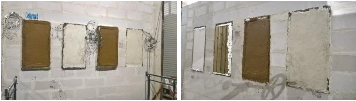
Fig. 2: Specimens placed on the vertical fire test wall: left: unexposed side, right: exposed side
