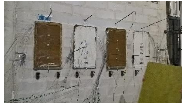
Fig. 4: Specimens with instrumentation before the fire test.
