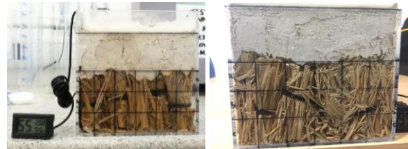
Figure 9. Specimen of wheat straw with perpendicular placing before the degradation research (left) and after 12 weeks in climatic chamber (right).
