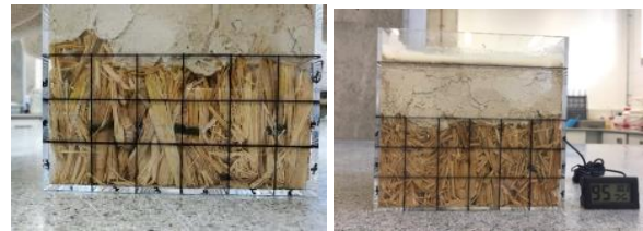
Figure 8. Specimen of rice straw with perpendicular placing before the degradation research (left) and after 12 weeks in climatic chamber (right).
