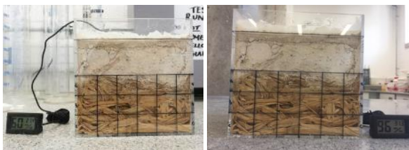
Figure 7. Specimen of rice straw with parallel placing before the degradation research (left) and after 12 weeks in climatic chamber (right).
