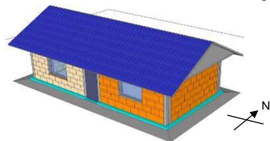
Figure 6. Perspective of the experimental building with laid flat straw bales (light yellow) and on edge straw bales (dark yellow).
