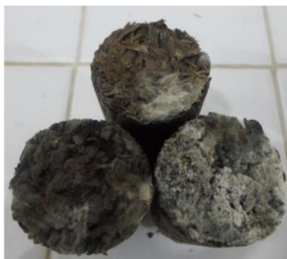
Fig. 5: Top of the WS 0.5 Samples after capillary test
