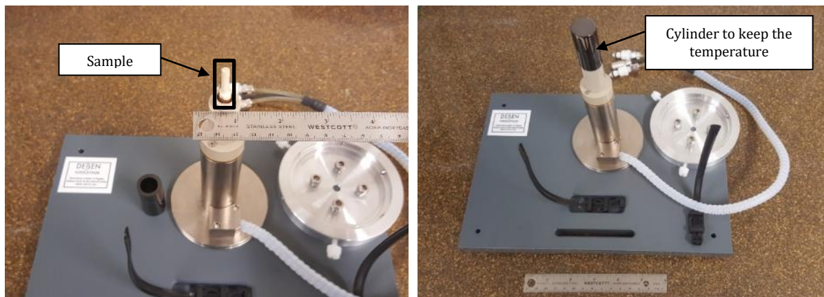
Figure 1. Tomographic stage for the generation of thermal flows
