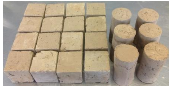
Fig 3: Cube and cylindrical specimen
