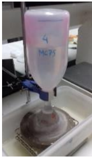
Fig. 94: Water permeability test.
