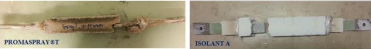
Figure 7. Failure modes of TRC5Mat-dI specimen protected by PROMASPAY@T and the insulator A
