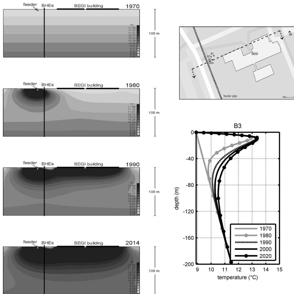
**Figure 4.** Ground temperature field evolution based on the numerical results.
