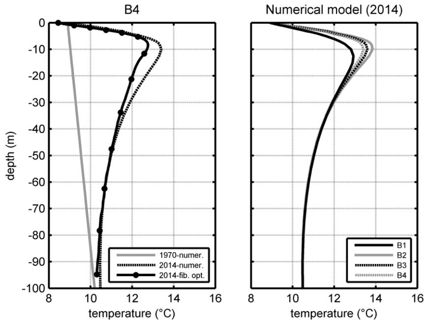
**Figure 5.** Experimental and numerical results of the ground temperature at the location of the four boreholes.
