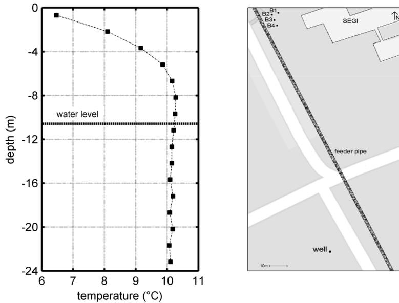
**Figure 3.** Undisturbed ground temperature measured by lowering a RTD probe inside the borehole well (24 February 2016).
