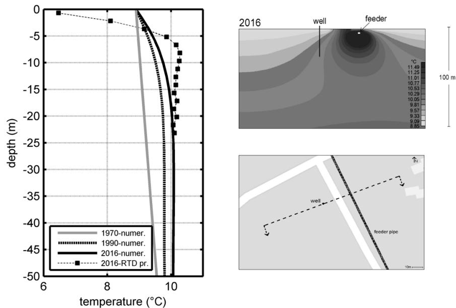
**Figure 6.** Experimental and numerical results of the ground temperature at the location of the well
