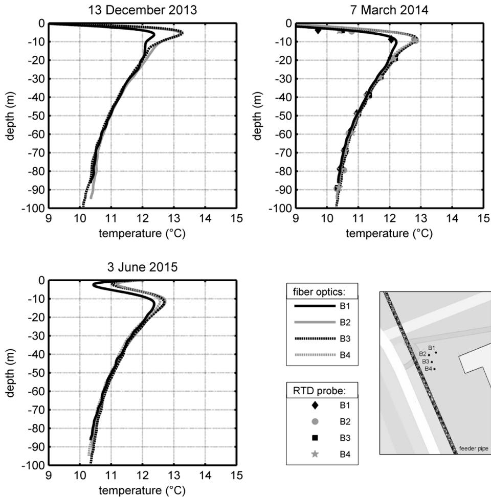
**Figure 2.** Undisturbed ground temperature measured by the fiber optics and by lowering a RTD probe inside the U-pipe in the four boreholes.
