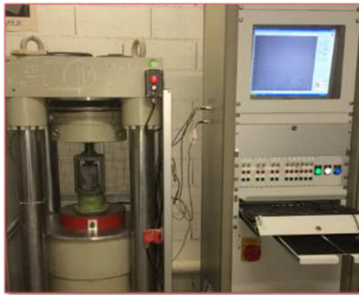
Figure 1. Experimental Set-up for the uniaxial compression test on \phi 110 \times h 220 mm specimen of concrete at 28 % aggregate volume fraction.
