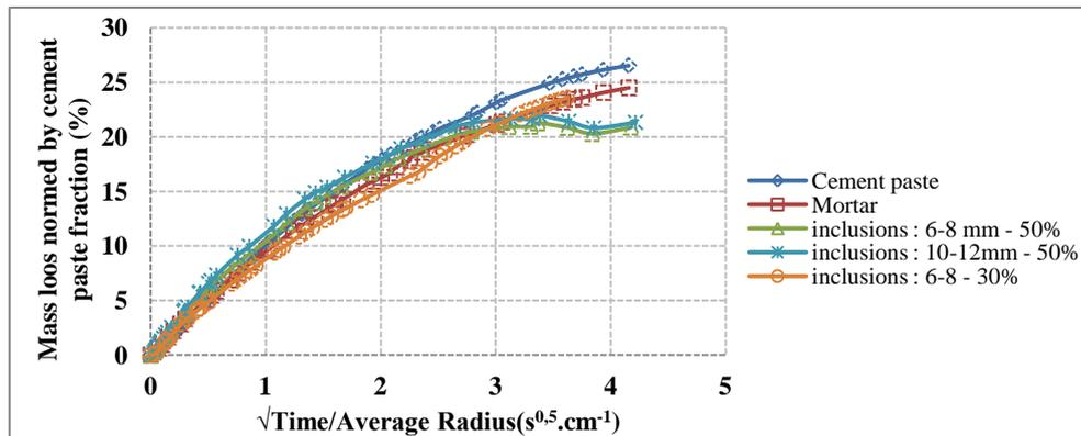
**Figure 3** - Evolution of mass loss normed by cement paste volume fraction with time under drying conditions
