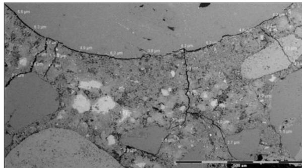
**Figure 1** - Low magnification image of a sample after drying at 105°C, displaying cracking induced by aggregates restraint. [WON 09]
