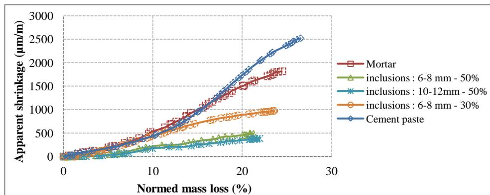
**Figure 4** - Total shrinkage of the studied compositions versus relative normed mass loss percentage under drying conditions
