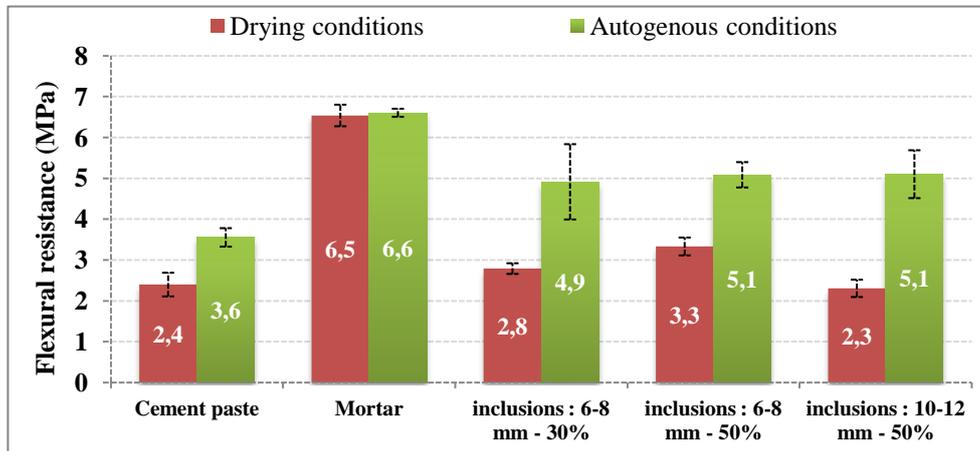
**Figure 5** – Flexural resistance of the different composition at the end of the monitoring in drying and autogenous conditions
