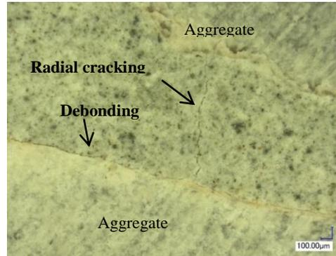
**Figure 7** – Observation of the cracking with a digital microscope
