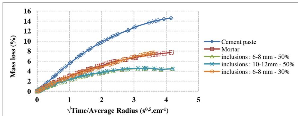
**Figure 2** - Mass loss evolution of the studied compositions with time under drying conditions
