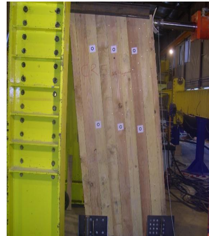
Figure 4: Timber cross plank wall in test.
