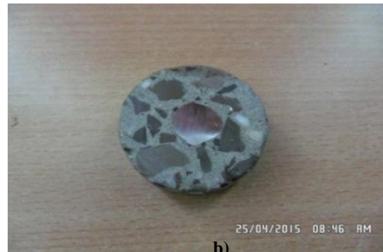
Figure 1: Rebar of steel type BE500S, a) of nominal diameter 16 mm and b) the same bar inserted into a 45 mm diameter concrete matrix used for the interfacial indentation test.
