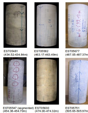
Figure 2: Cores taken from the Callovo-Oxfordian argillite at MHM- URL
