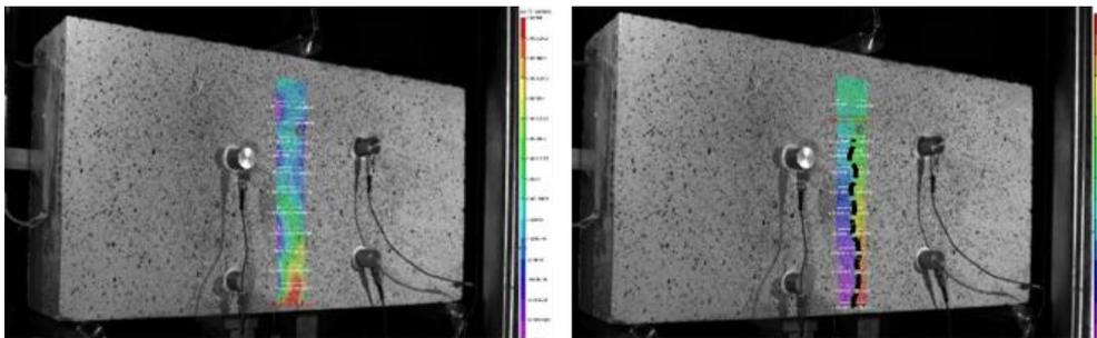
**Figure 6.** a) Strain distribution, b) Crack way and opening
