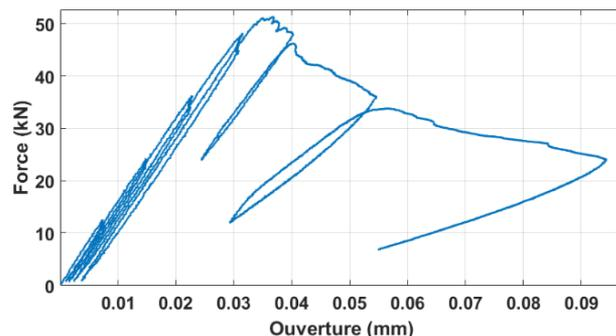
Figure 2. Force-CMOD curve.
