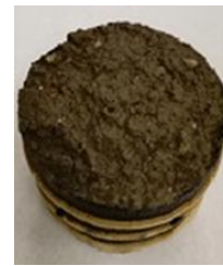
Figure 4. Swelling after 7 days curing period
