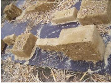
Figure 2: Adobes fibrés (1200 kg/m<sup>3</sup>)
