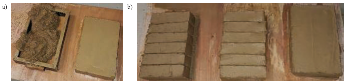
Figure 1. Construction of specimens: a) casting earth into mould, b) specimens after wire-cutting.
